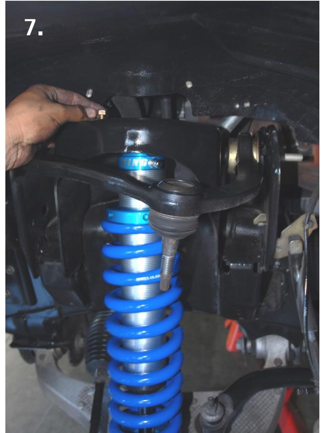
Once the shock is in place reinstall ball joint mount and tighten all nuts.
