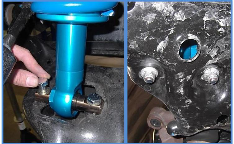
16. For Remote Reservoir Shocks: Route the hose behind the fender liner and position the reservoir in the reservoir bracket. Use the provided hose clamps to secure the reservoir to the reservoir bracket.
