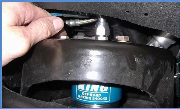
15. Line up the lower mount and use the supplied 12mm bolts and washers along with the factory nuts. Install hardware but do not tighten yet.
