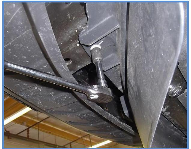
8. Open the hood to access the hood latch bolt and two other bolts that need to be removed. Use a 10mm socket for the hood latch bolt and an 8mm socket for the other two bolts. Also, make sure the hood latch cable is unclipped from the fascia.
