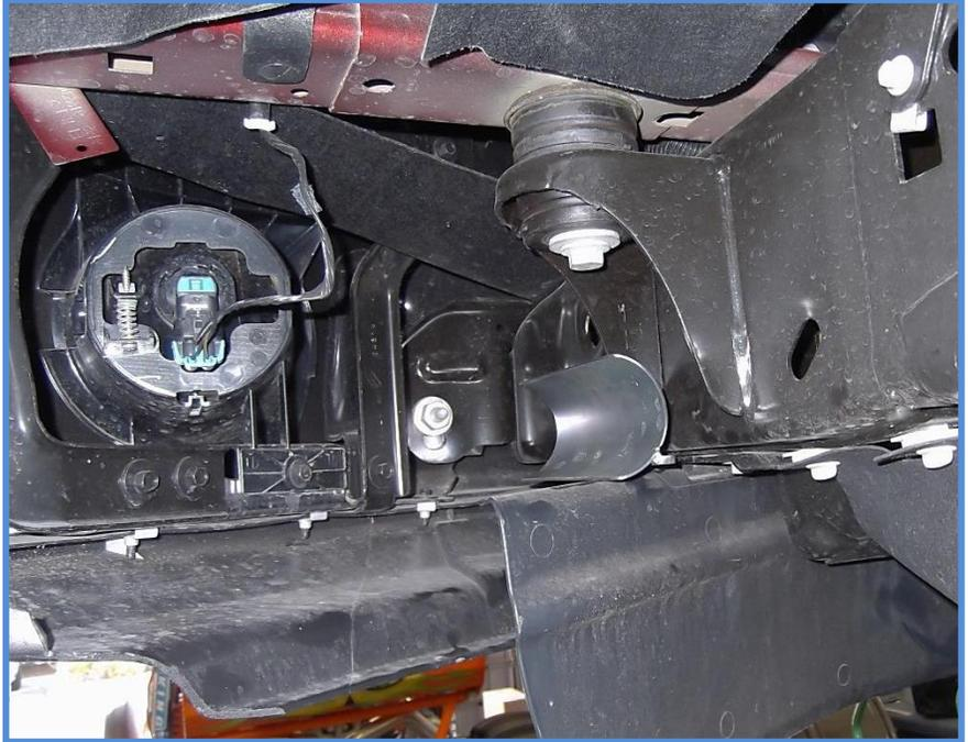
13. Install King Remote Reservoir Shocks by first feeding the reservoir through the hole at the top of the shock mount. Be aware that the shocks are side specific, the reservoir will route towards the front of vehicle as shown in the photos below.
