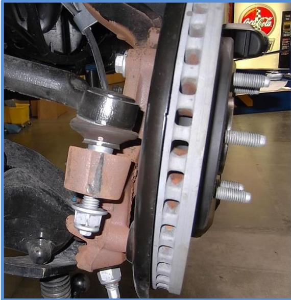
3. Disconnect the upper A-arm from the upright. Using a 21mm socket, loosen the nut on the A-arm ball joint. Separate the ball joint from the upright using proper ball joint tools.
