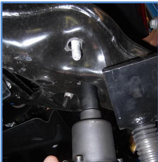
5. Using a 15mm socket, remove the three nuts from the top of the shock assembly and remove the shock.
