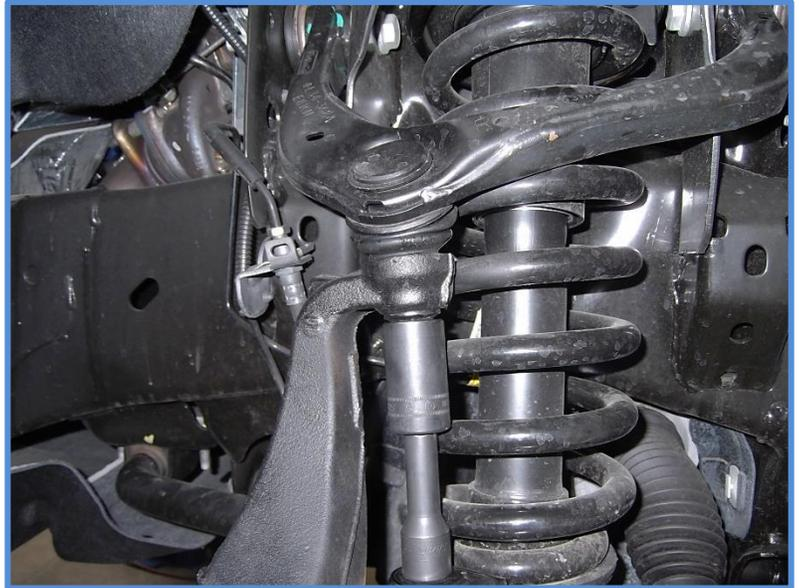
4. Remove the nuts from the lower shock mount using an 18mm socket. Save the nuts you will reuse them to mount the King Shocks.
