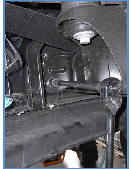
11. With the bumper removed you can now access the tow hook holes in the frame. Position the reservoir mount on the frame (as shown in the photos below) and install using the supplied 10mm hardware.
