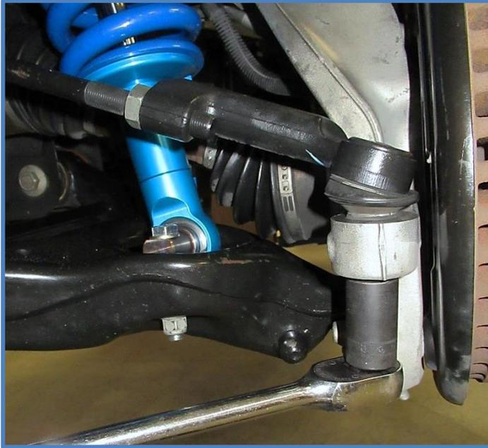
14. Reconnect the brake line/ABS line brackets.
