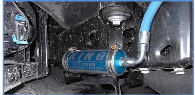
11. Using a 9/16" socket, torque the 3/8" upper shock mount bolts to 35ft/lbs. Torque the lower shock bolts to 75ft/lbs. using an 18mm & 19mm wrench/socket.
