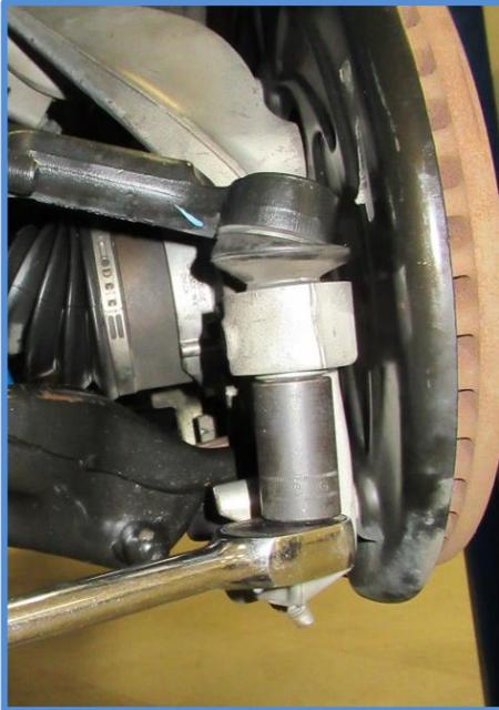
3. Disconnect the upper A-arm from the upright. Using a 21mm socket, loosen the nut on the A-arm ball joint. Separate the ball joint from the upright using proper ball joint tools.
