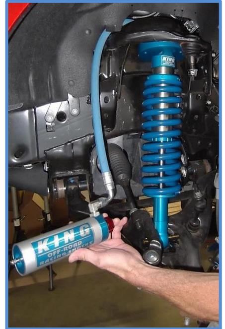
8. Line up the holes in the upper mounting plate on coilover with the upper mount on the vehicle and use the supplied 3/8" bolts and washers to attach the new coilover to the factory upper mount. Thread the bolts in enough to hold shock in place but do not tighten yet.
