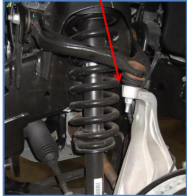
4. Remove the nuts from the lower shock mount using an 18mm socket. Save the nuts you will reuse them to mount the King Shocks.
