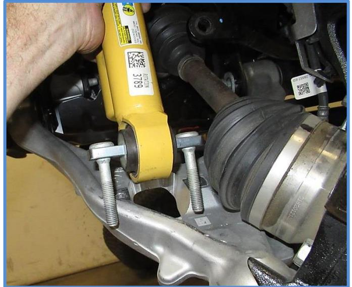
Place the lower control arm back into the lower mount and install the cam bolts to the same position prior to removal and tighten to factory specs. The vehicle will need to be aligned properly after the install but keeping the factory settings will get you to the alignment shop.
