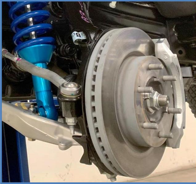
12. Reconnect the upper control arm and tighten to factory specs.
