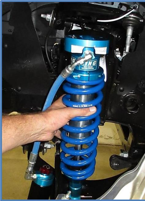
9. Install the provided 3/8" upper mounting bolts (CB4701) with HD washers (CW1701). Thread the bolts into the upper mounting plate to hold shock in place but do not tighten yet.
