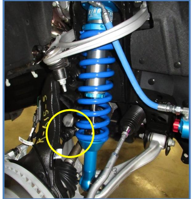
16. Mounting reservoirs – First attach the reservoir clamps to the reservoir brackets. Use the 1/4 X 1/2" BHCS (CB2420) to attach the reservoir clamps. Photos below show bracket for right side of vehicle. For the left side of vehicle mount clamps on opposite side of plate.
