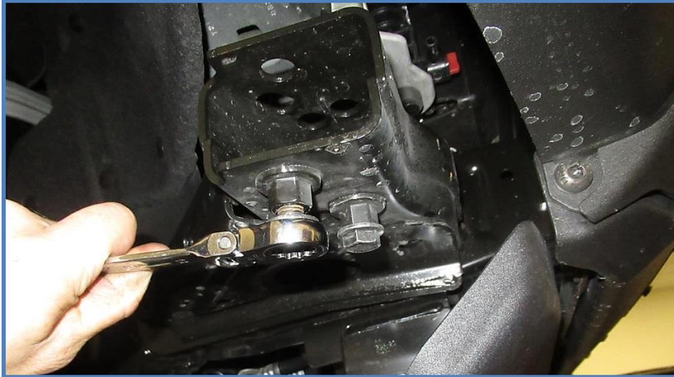
18. Slide the reservoir into the reservoir clamps then place the bracket on the front cross member and reinstall the two factory bolts.
