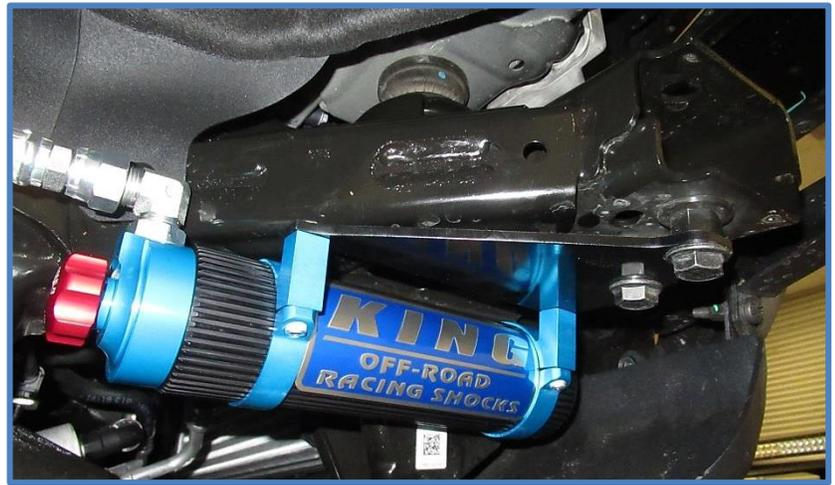
19. Install the 1/4 X 1" bolts (CB1501) in the reservoir clamps and tighten using a 3/16 Allen wrench.
