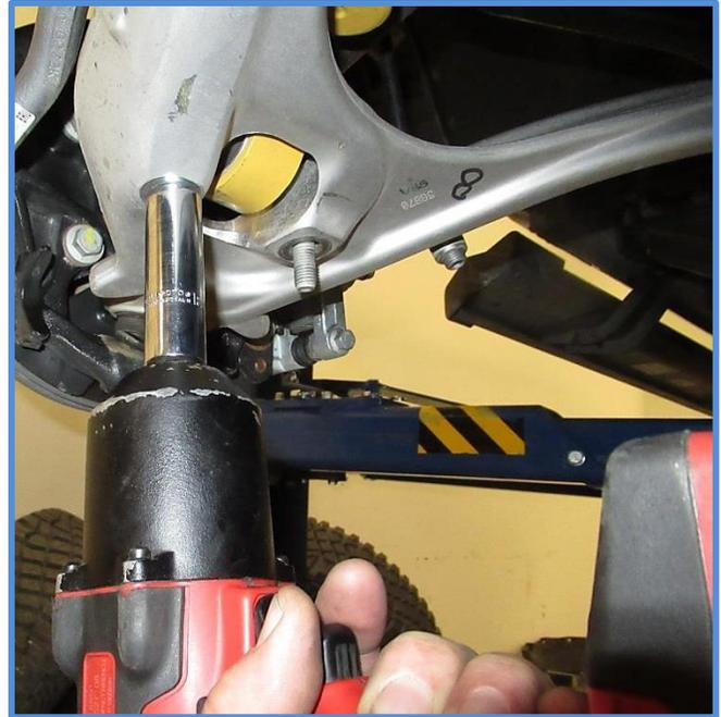
4. Separate the upper control arm from the knuckle. Using an 18mm wrench or socket remove the nut for the control arm ball joint, then disconnect upper arm from knuckle.
