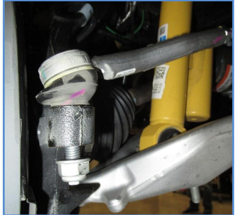
6. Disconnect the sway bar links on both sides of the vehicle. Remove the nut using a 21mm wrench, you may need to hold the stud with a hex key to keep the stud from spinning.
