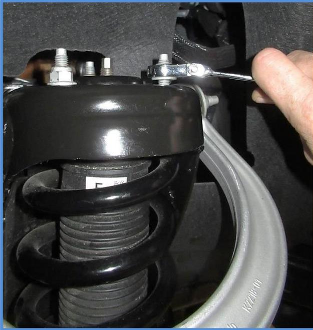
3. Remove the lower mounting nuts using an 18mm wrench or socket.
