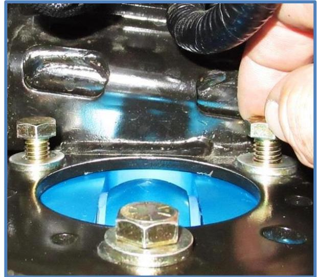
10. Install the provided 12mm X 80mm bolt (CB3829) with washer (CW1001) through the lower mounting lug and lower control arm. Place the reducer sleeve over the bolt and then install the factory nut. Thread the nut onto the bolt but do not tighten yet.
