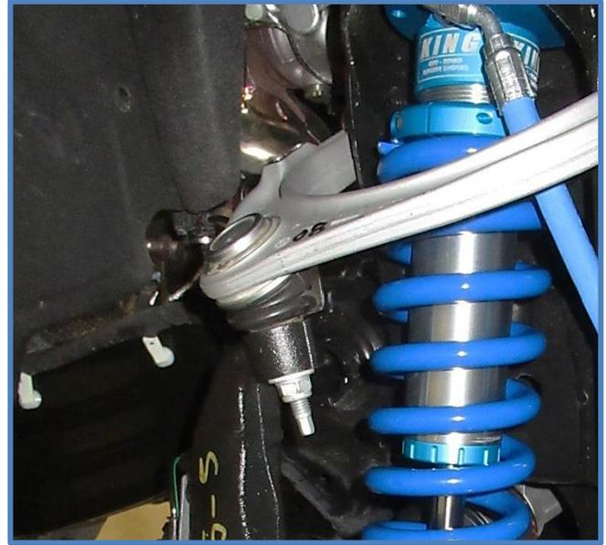
13. Now you can torque the upper and lower mounting bolts. Torque the upper bolts to 35 ft/lbs. using a 9/16 socket. Torque lower bolts to 90 ft/lbs. with an 18mm socket on the nut & 19mm wrench on the bolt head.
