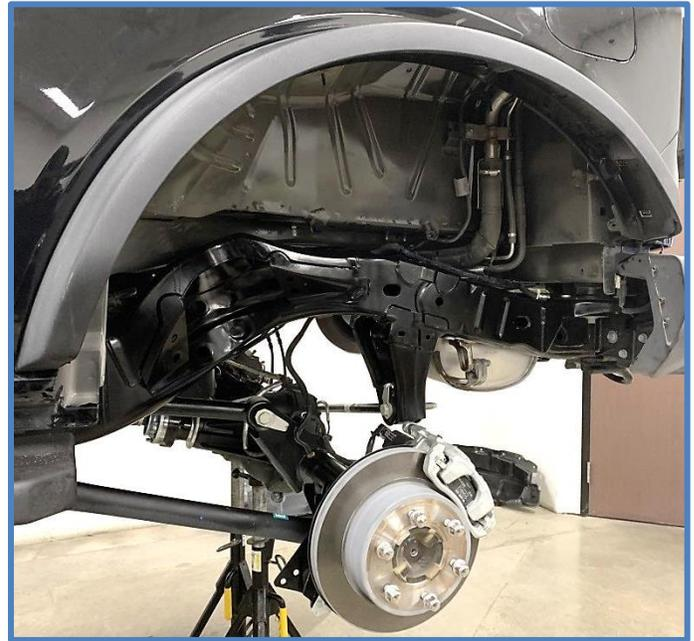
3. **Install King Shocks** – Be aware the shocks are side specific, make sure you are installing shocks on the proper side. See final install picture for reference. Place the shock into the upper mount and install the 3/8 Heavy Duty washers (CW1701) and 3/8 nuts (CN2711) on upper mounting studs and tighten nuts to hold shock in place but don't fully tighten yet.
