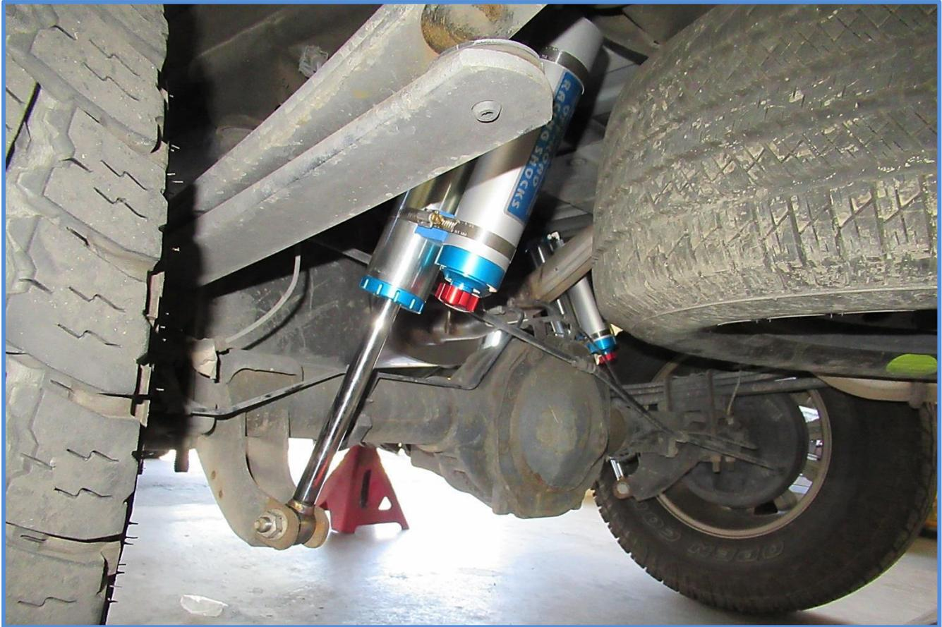
**Make sure shocks are installed properly and all hardware is tight. Remove jack stands and lower vehicle. Double check all hardware after 100 miles or so and periodically after that as part of routine maintenance.**
