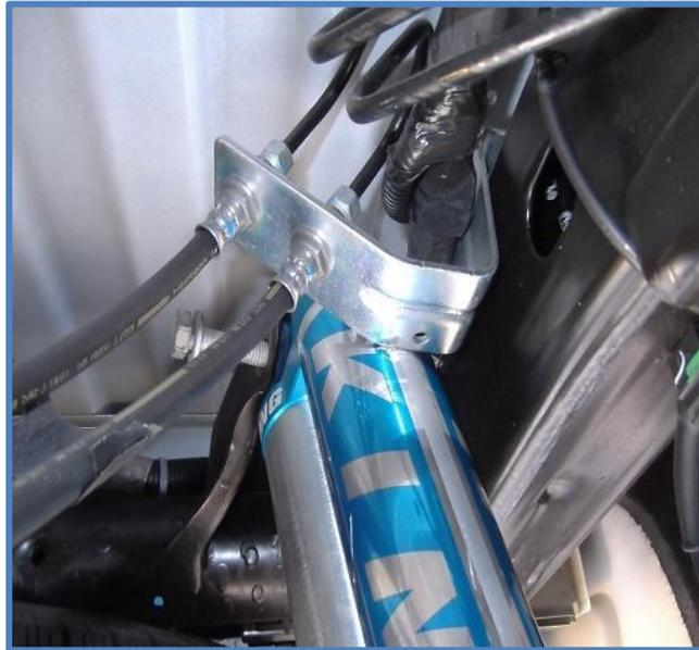
3. **For shocks with Compression Adjusters:** Shocks with compression adjusters need to be mounted so that the reservoirs are both facing towards the rear of the vehicle. Use factory hardware to install shocks and torque to factory specs.
