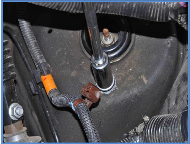
3. Loosen the nut for the ball joint on the upper control arm and separate control arm from upright but do not fully remove yet.
