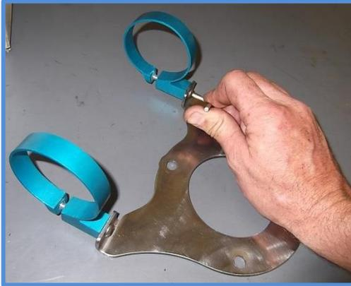
8. Slide the reservoir bracket over the reservoir as shown below.
