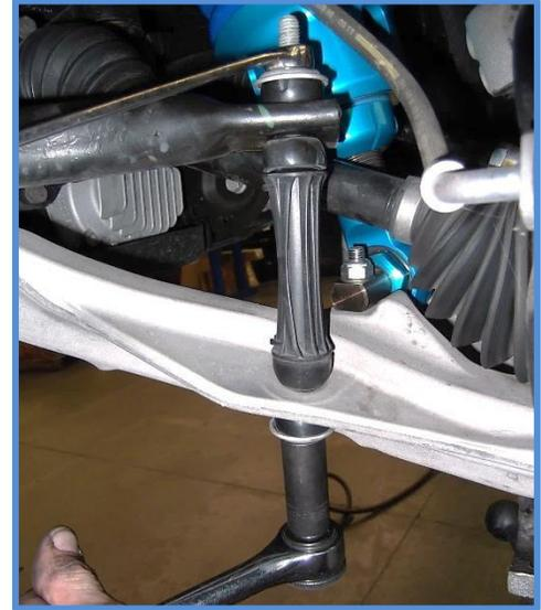
12. Pay special attention to brake lines, ABS lines etc. Make sure you have enough slack at full droop and full turn. Make sure there are no interference/clearance issues or lines that can get caught on moving parts.
