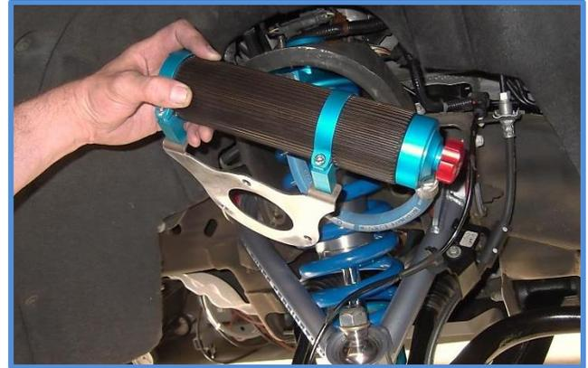
9. Place a jack under the lower control arm and jack the arm up until the upper mounting plate is tight against the coil bucket. Place the reservoir bracket over the studs and install the provided 3/8" washers and nuts and tighten. Now tighten the lower hardware, with all the hardware tight you can lower and remove the jack.
