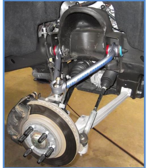
6. Install King Shocks. Shocks are side specific, be sure you are installing the shocks on the proper side. Place the shock in position on the vehicle and install the 10mm lower mounting bolts w/washers, nuts provided in the kit but do not tighten.
