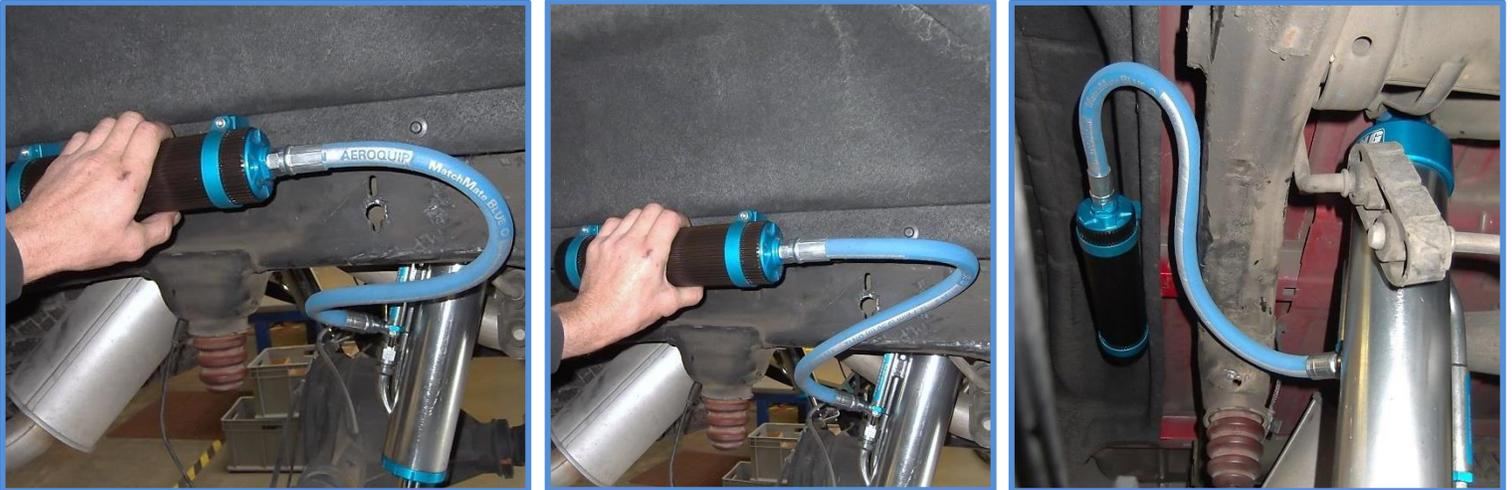
14. Once the reservoirs have been secured in the final position you can attach the KING nameplate. Be sure to clean the reservoir with alcohol. Peel the adhesive backing off the back side of name plate and place the plate on the reservoir. Use zip ties to hold the plate tight to the reservoir for at least 72 hours. Zip ties can be removed after 72 hours. **(3M recommends a 72 hour cure time for maximum bond strength)**
