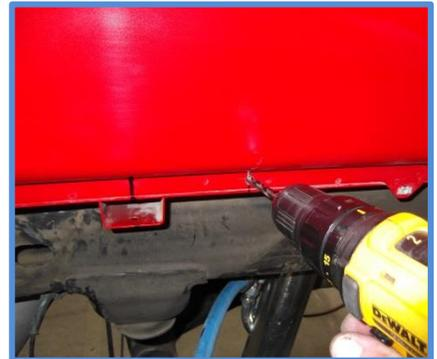
6. Place the fender liner back in position on the vehicle to mark for drilling but don't screw back in yet. Mark the two holes, remove from vehicle and drill 1/4" holes. Place the fender liner back on the vehicle, make sure the holes are lined up. Replace all the screws and tighten.
