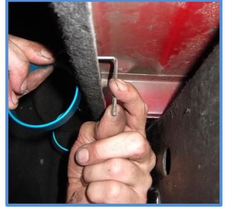
8. Place the reservoirs in the clamps. Starting with the left side, loop the reservoir into the clamps as shown.
