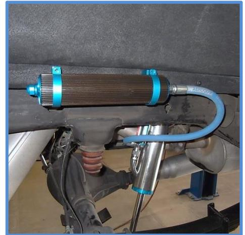
12. Install the 1/4 x 1" socket cap screws and snug so the reservoir can still be rotated in the clamps.
