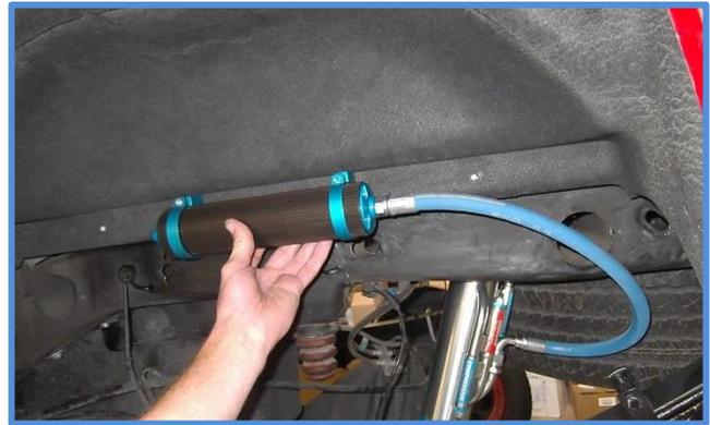
9. Use the provided loop strap, fender washers and 1/4 x 1" bolt with nut to hold the hose to the frame. **(Left side only)** Place loop strap on hose, place oval washer in the recessed oval hole in the frame. Use the 1/4 x 1" bolt and nut with fender washer on the back side of frame to attach hose. This step is important to make sure the hose does not rub on tire and leaf spring.
