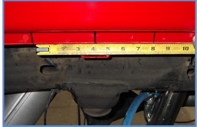
5. Find the center of the two outside lines and use a center punch to mark the location for drilling. Drill 1/4" holes.
