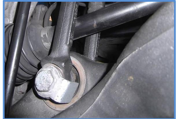
13. Now with the floor jack still under the lower control arm raise the jack until the weight of the vehicle is on the suspension and the frame just starts to lift off of the jack stand. With the weight of the vehicle on the suspension you can tighten all hardware, start with the 4 upper bolts, then tighten the clevis/strut fork bolt and finally the lower mounting bolt.
