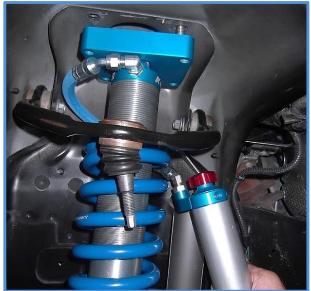
11. Place the factory clevis/strut fork on the lower end of the King Shock and insert the factory bolt with the ABS line bracket included in the kit as shown in the photo's below. **DO NOT TIGHTEN**.
