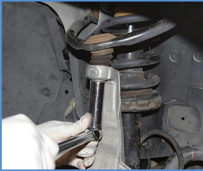
4. Remove the bolt from the strut fork Clevis at the bottom of the shock body using a 21mm socket.
