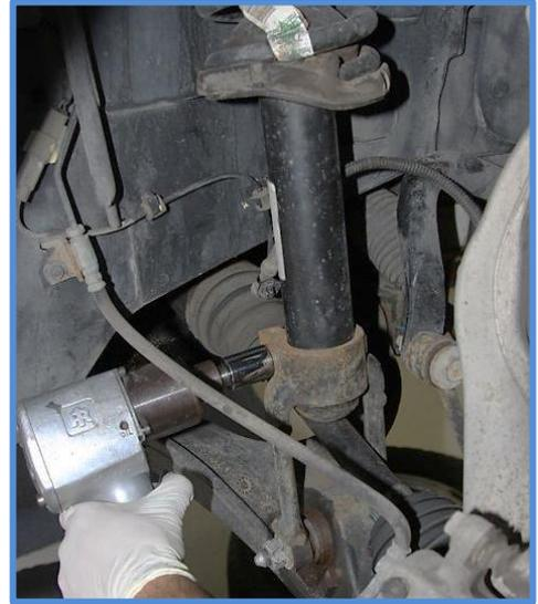
5. Remove the nut from the lower mounting bolt using a 24mm socket. After removing the bolt you can lower the jack so the shock is free hanging and clear of the lower control arm. Pay attention to the ABS and brake lines as you do this to ensure the lower control arm and steering knuckle are not hanging by these lines.
