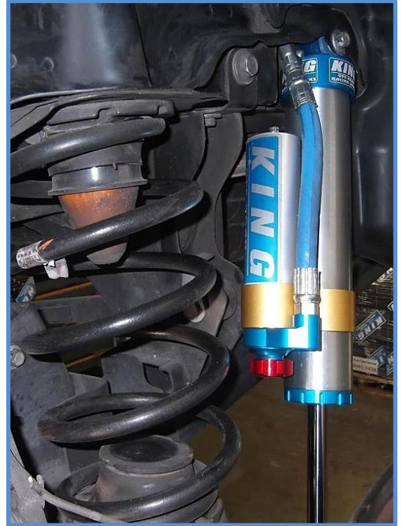
Make sure everything is installed correctly and all hardware is tight before reinstalling tires. Install tires, remove jack stands and lower vehicle to the ground. Recheck all hardware and lug nuts after 100 miles and periodically after that as part of routine maintenance.
