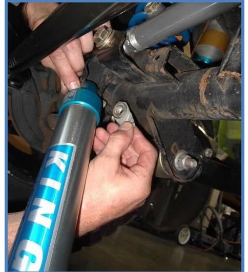
6. Install steering stabilizer on tie rod bracket. Install 3/4" spacer first, then steering stabilizer followed by the small spacer and nut. Tighten nut with 18mm wrench/socket. Photos below show the steering stabilizer mounted to the tie rod bracket.
