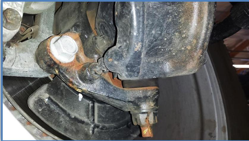
**Double check your install, make sure the stabilizer is mounted properly and all hardware is tight. Recheck the hardware after 50 miles and periodically after that as part of routine maintenance.**
