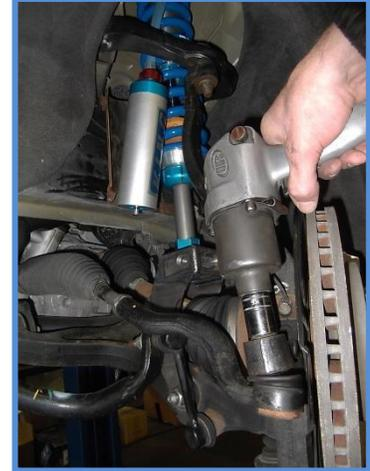
14. Place reservoir in the cradle and install hose clamps, position reservoir so the hose does not contact upper control arm.
