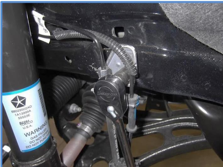
2. Disconnect the sway bar using an 8mm wrench to hold the stud and an 18mm wrench to remove nut.
