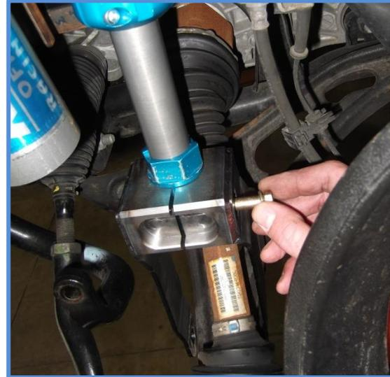
11. Attach Clevis to the lower control arm using the factory bolt but do not tighten yet.
