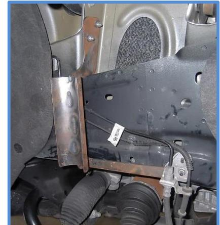
9. The King Shocks are side specific, be sure the shocks are being mounted on the correct side. (The hose should be towards the front of vehicle) Having someone hold the shock in position while someone else is starting the upper mounting bolts is the easiest way to install the coilover. Get the upper mounting bolts started to hold the shock in place first but don't fully tighten yet.
