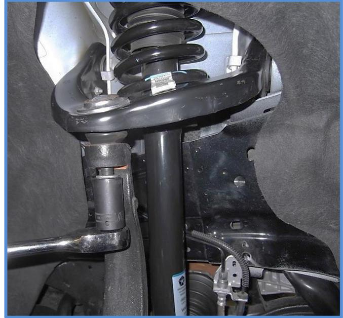
5. Remove the lower shock mount bolt using a 21mm socket on the bolt head and a 24mm wrench on the nut.
