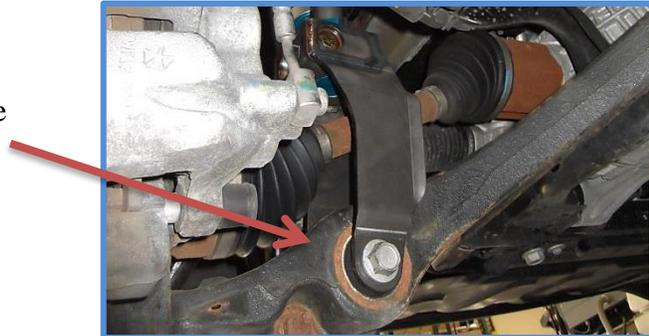
12. With all of the hardware installed but not tightened yet, jack up the lower control arm so that the weight of the vehicle is on the suspension to the point where the frame is coming off of the jack stands. Now you can tighten the **three upper mounting bolts**, the **clevis pinch bolt** and the **lower OE shock mounting bolt**.
