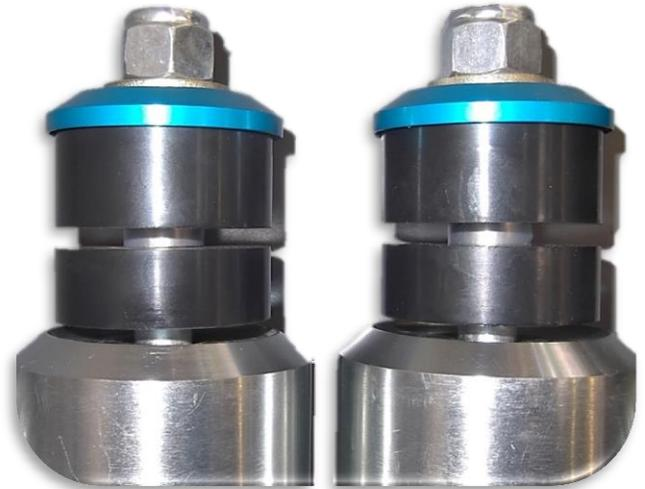
3. For the lower mount place one spacer on the mounting stud (A), then install the rod end followed by the other spacer. Make sure that the spacer is not sitting past the mounting stud (B). Use the factory bolt and tighten to factory specs (C). See photos on next page for proper shock orientation, position shocks accordingly and tighten the nut on the upper mount.
