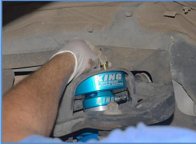
4. Install the factory bolt in the lower mount and tighten to factory specs. You can now tighten the three upper mounting bolts also.
