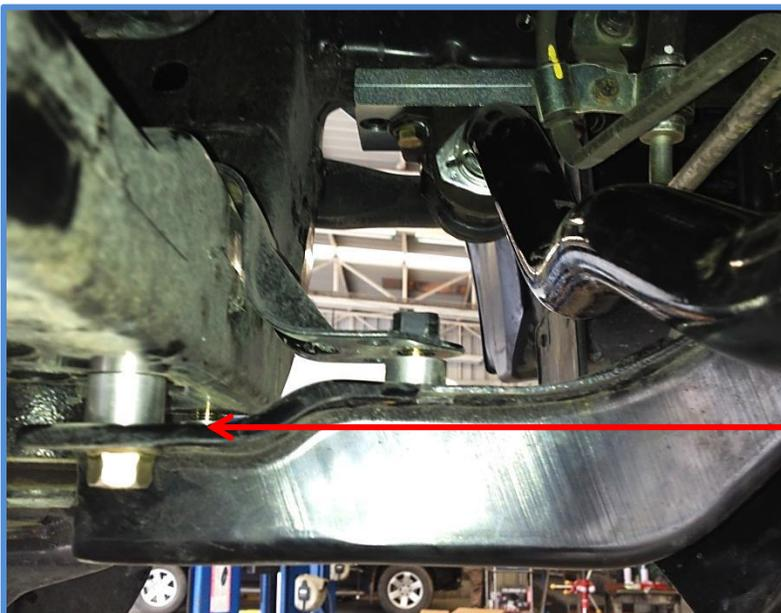
**Photo shows an example of spacers installed to lower the skid plate support brackets providing clearance for sway bar.**
