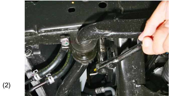
(2) Remove the sway bar end link from the spindle. Remove the bolts holding the sway bar to the chassis.
