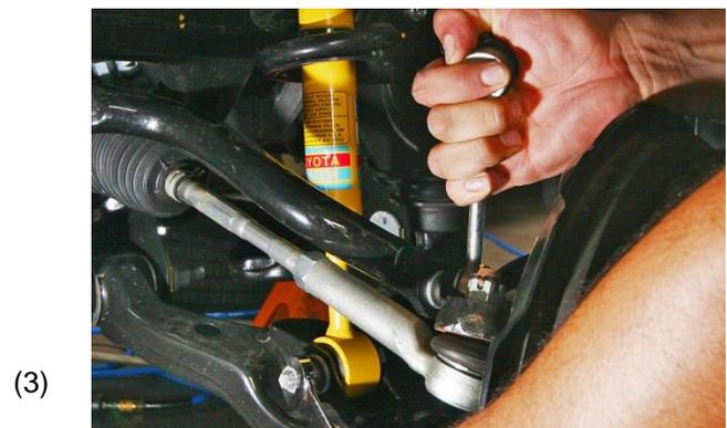
(3) Remove the nuts from the upper and lower shock mounts but leave the bottom bolt in for now.
