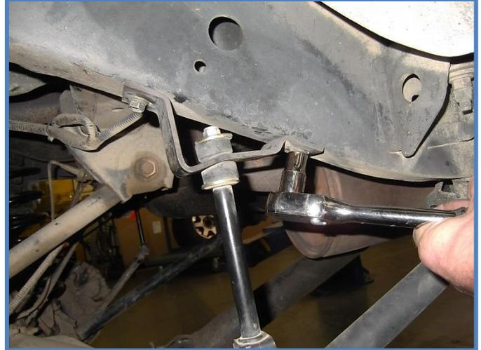
3. Place brackets in position on the frame lined up with the sway bar mounting holes. Brackets are side specific, be sure to mount brackets on the proper side (see photos below - Photos show right side being installed). Use the OE bolts you just removed to bolt the sway bar bracket back in place over the reservoir bracket.
