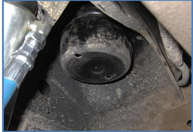
3. Using a 2 1/4" hole saw, cut a hole in the center of the bump stop mount using the threaded hole in the center as a guide for the pilot bit.
