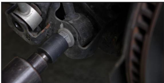
8. Bolt the reservoir bracket between sway bar mount and frame using the factory hole locations and factory bolts. Check fit and tighten.
