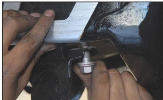
6. Next remove the front skid plate. This is necessary to gain access and remove the sway bar. You may need two people to help hold skid plate for easy removal.
