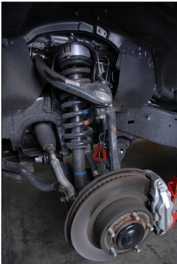
With the vehicle on level ground, set the emergency brake and block the rear tires. Using a floor jack, jack up the front end and support the frame rails with jack stands for safety. Then remove the front tires.
