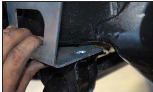
5. Using a 22mm socket, remove the lower shock mount bolt. The lower shock mount bolt may be difficult to remove so use an oil lubricant and a long punch to remove the bolt. Next remove the sway bar from lower A-arm by using a 19mm socket. As always be careful not to damage the bolt or the threads.
