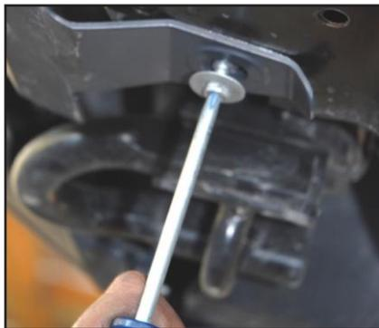
9. Slide the King coil over in bottom first then push up on upper a-arm. Slide the shock into the upper mount. Start the four 3/8 x 1 inch bolts to hold the shock in place but don't tighten. Line up the lower mount and slide the bolt through (you might need help pushing down on the lower a-arm). Now starting up top, tighten all the bolts.
