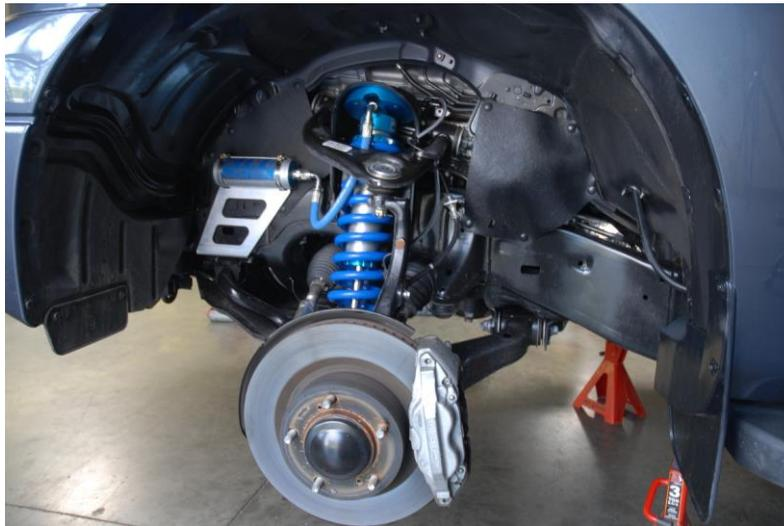
Reconnect A-arms, sway bar links and brake line brackets. Install the reservoir in the reservoir bracket using the supplied hose clamps. Make sure the reservoir hose is routed as shown and does not rub on the moving parts of the suspension. Reinstall the skid plate and check to make sure all your bolts are secure and tightened. Reinstall tires.
