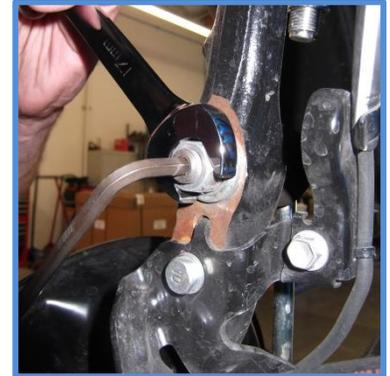
Use an allen wrench to hold the sway bar link stud for removing and tightening nut.
