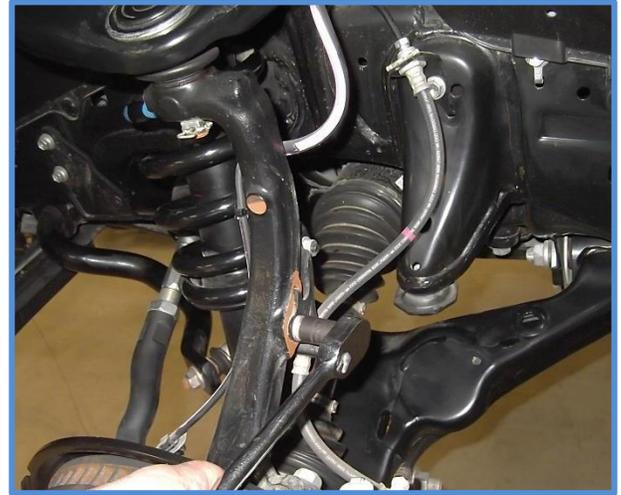
4. Pull the pin out of the ball joint stud in the upper control arm using needle nose pliers.
