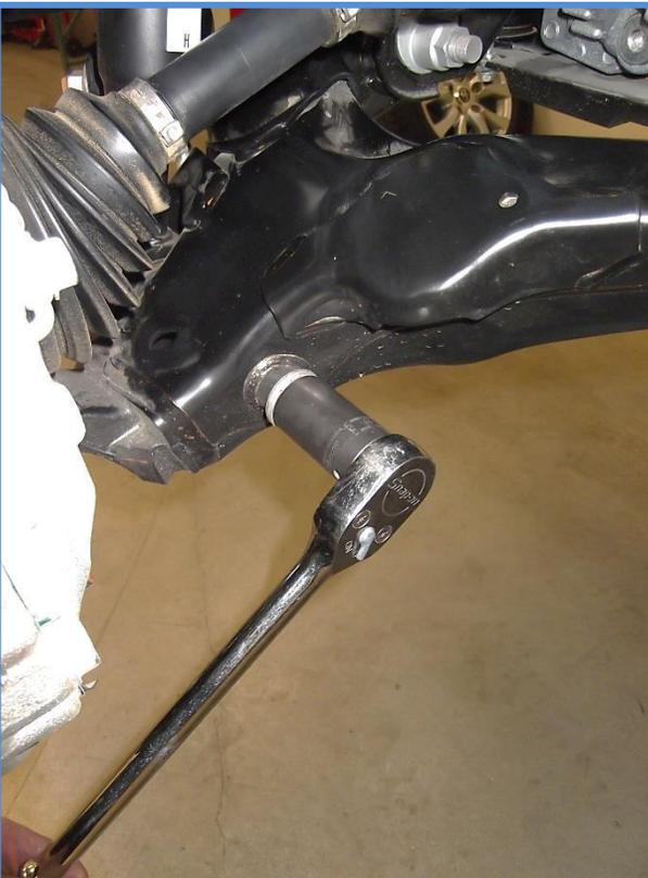
9. Once the factory shock has been taken off the vehicle, unbolt and remove the factory upper control arm by removing the long through bolt located behind the coil bucket. Install the King Coilover with the control arms removed then install aftermarket arms as per the instructions that came with your control arms.
