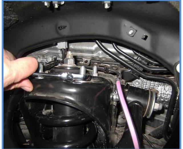
8. Remove the lower mounting bolt using a 22mm wrench and socket. Remove factory shock.
