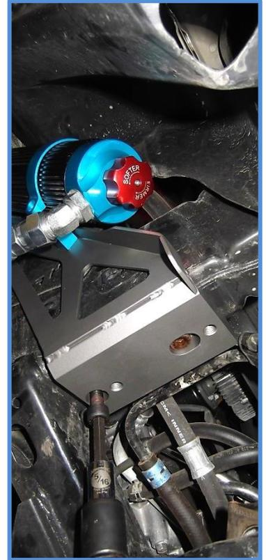
23. Bolt the sway bar to the bottom of the reservoir bracket using the supplied 3/8 X 3/4" bolts (CB4702). Tighten bolts to 35 ft-lbs. Repeat steps 20-23 on opposite side of vehicle. Reinstall skid plate after both sides are done.
