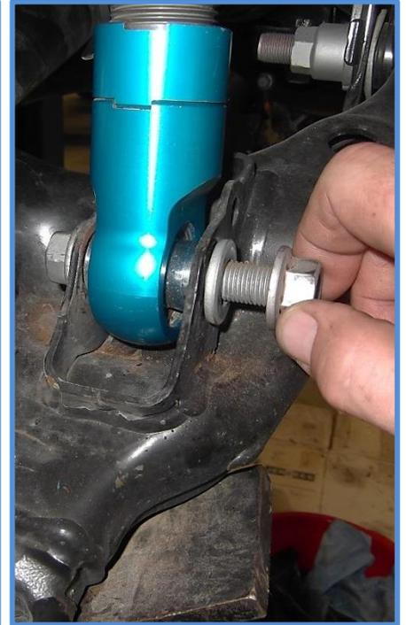
12. Jack up the lower control arm so the upper mounting plate is tight against the upper mount and install the 3/8 HD washers (CW1701) and 3/8 nuts (CN2711).
