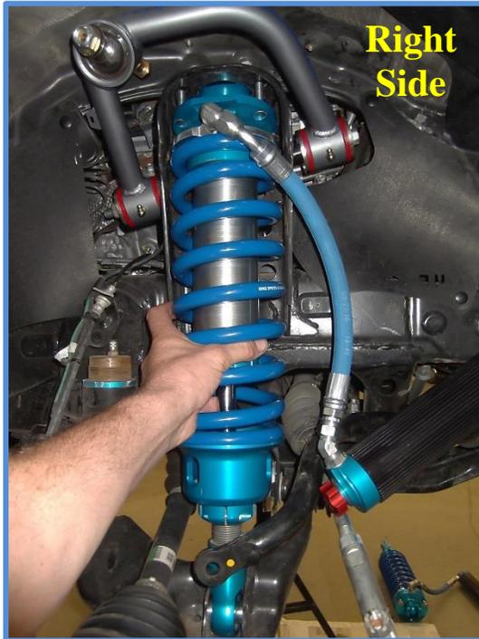
11. Install the factory lower mounting bolt in the lower mount as shown below. Place the washer and nut on the bolt but leave loose for now.
