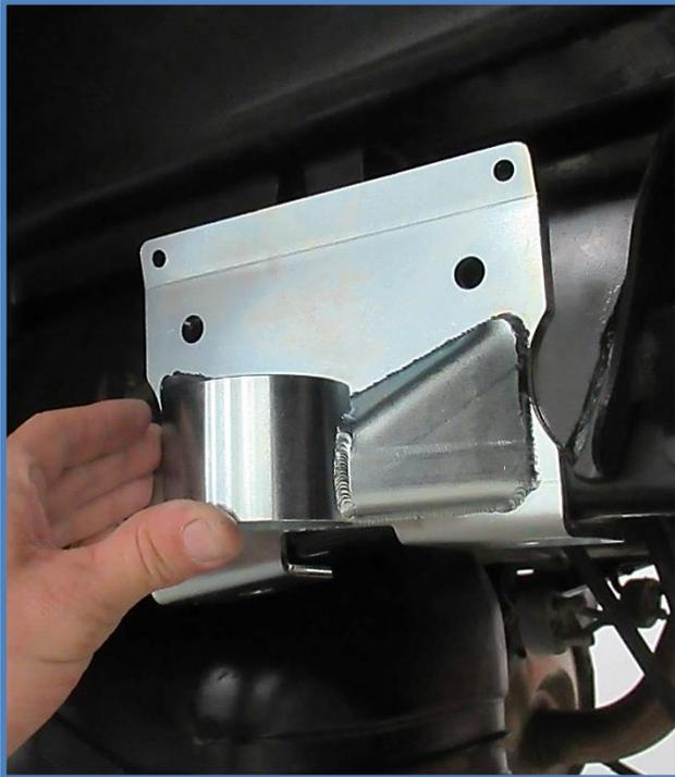
3. Install the 7/16 X 1" bolts (CB4601) with washers (CW1001). It may be necessary on some vehicles to enlarge one or more of the holes in the frame to install hardware.
