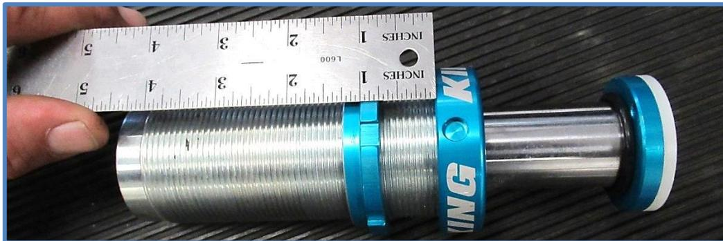
8. Now place the bump stop in the bracket and thread the upper lock ring onto the bumpstop.
