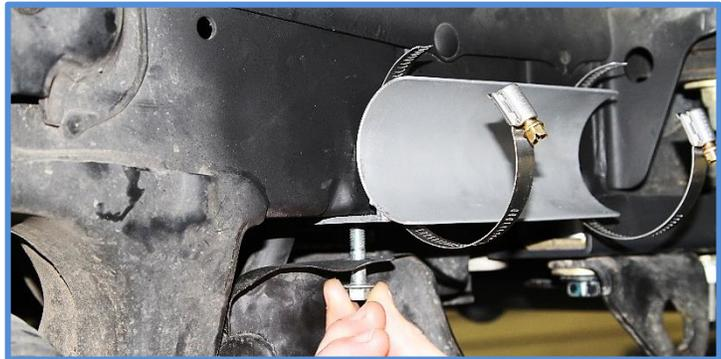
6. The reservoir mounts with hose fitting pointing up. Make sure hose does not interfere with moving suspension parts. Install hose clamps as shown, tighten clamps then tighten remaining bolts.
